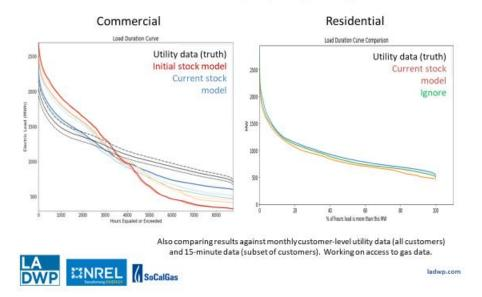
Once we build these models, we need to calibrate them using utility data. The left graph shows how the initial stock model (in red) does not reflect the actual utility data (in black). By going through and calibrating the models we are able to bring the models much closer to actual data, although they still do not match exactly. The residential model came out much closer after calibration. All this is for electric, we still have to do the gas side.
